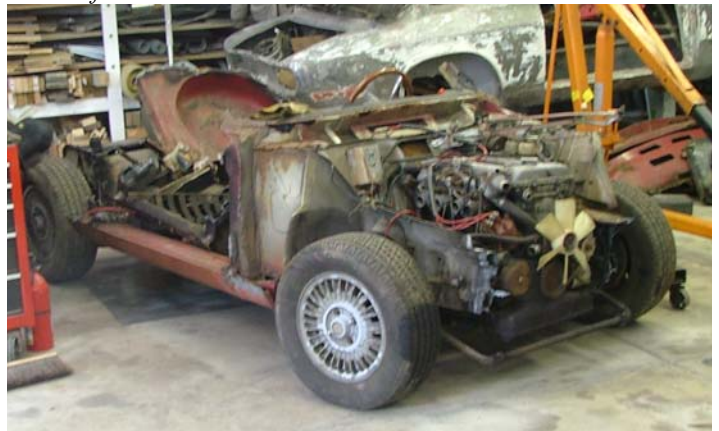
With the roof and rear clip removed, it’s looking svelte. I am always amazed at how little structural support the roofs of GTVs have. I hope never to roll one.
