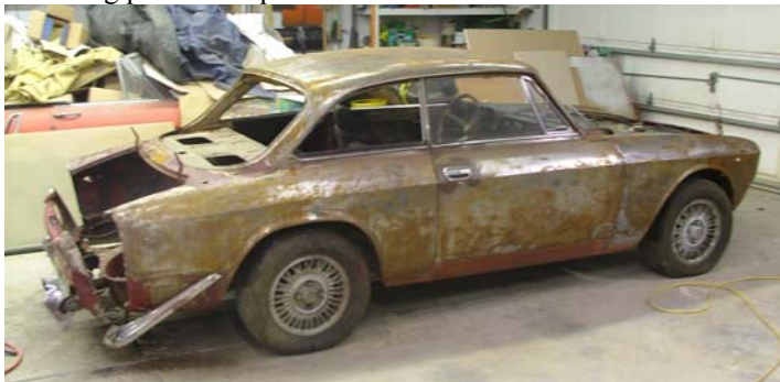
Almost as it arrived, the rear valance has just been severed.
