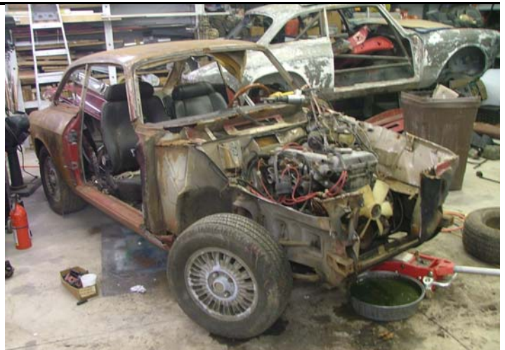
The next step was to remove the front valance and wings. I was surprised how easily the spot welds broke away with the air chisel. Note the “rivet queen” in the back, spared from the torch... for now.
