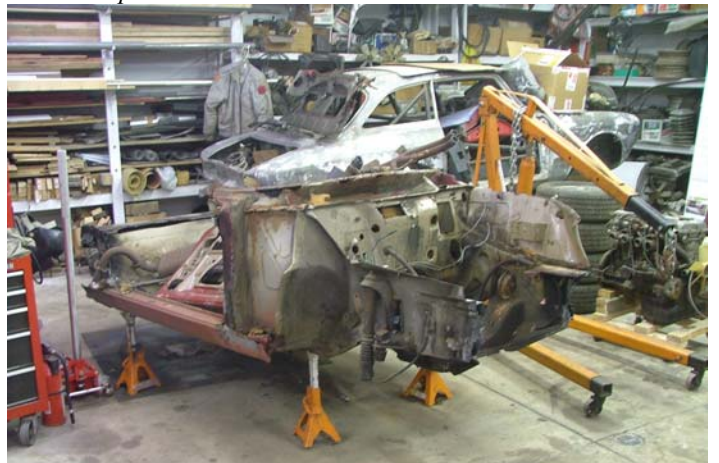
With drivetrain, all the mechanical and interior parts removed, the remaining steel structure is ready for the junk yard. Fortunately, a guy I work with has a brother-in-law who owns a junk yard, and was willing to take the shell. Last time I did this, I had to chop it up into sizes small enough to put in the trash can. It also takes a while to get rid of the pieces that way.
