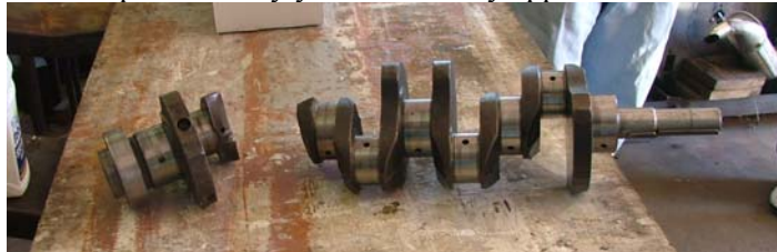
The famous two-piece Alfa Romeo crankshaft.
