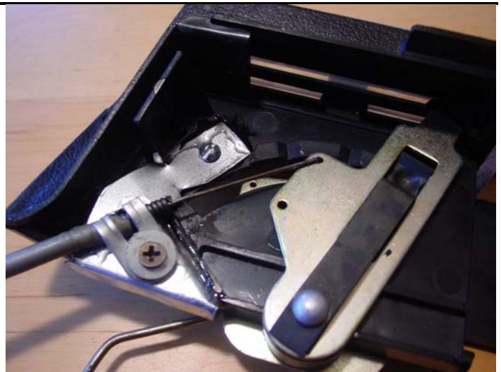
A little sheet metal, a little epoxy and the brittle Italian plastic bits are better than new
