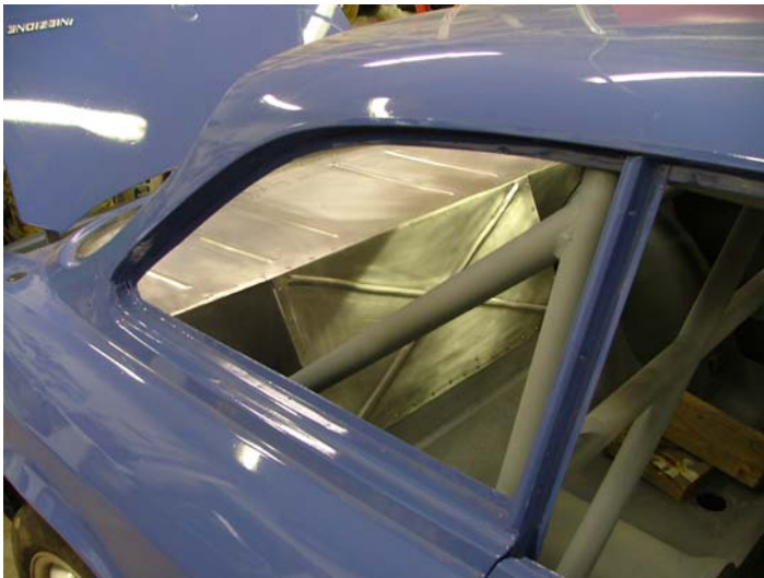
The finished aluminum rear bulkhead. Note the beading.
