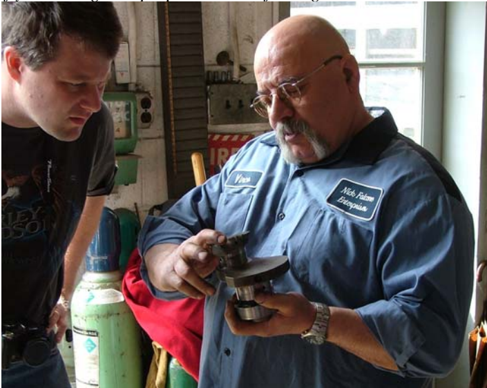
John Angeleri's son pays close attention as Vince points out the detail that was left out of this crankshaft, which caused it to crack in half.
