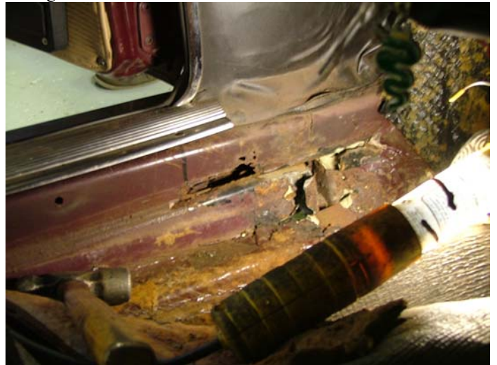
The driver's floor of Jack's GTV, not pretty, but nothing a little welding can't fix
